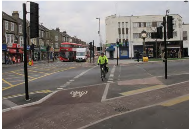
Figure 10.26: Circulating Cycle Stage Junction, Waltham Forest
